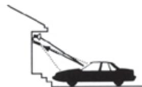
**Solution:** Aim sensor away from lights and reflective objects or mask the lens in the direction of the light or reflection.
