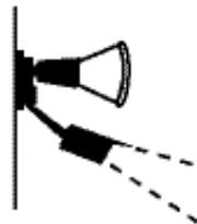
5. Make sure lights are not visible from or reflecting back into sensor. Check for white or reflective surfaces close to the sensor.
