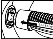
5. Rotate LED lamp until lamp locks in place. Ensure that the LED lamp front points away from the back of the luminaire.
