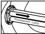
4. Bring LED lamp to luminaire and insert lamp pins into luminaire lamp holders.
