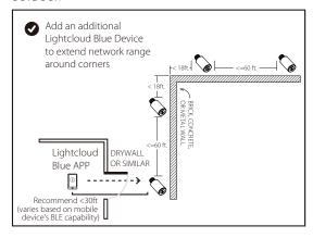
To enhance the mesh stability, customer can choose a suitable place to add the extra LCBLUECONTROL/B with junction box.
